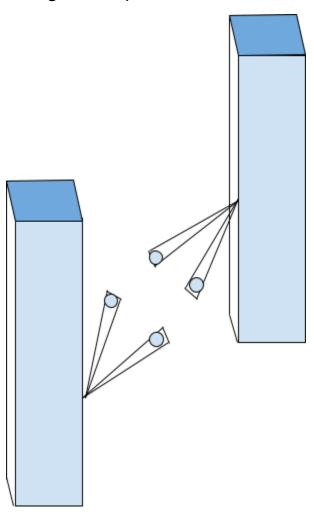
For this design, 2 posts will be fabricated as well as 4 mounting arms that will mount to the structural strong points of a vehicle such as its subframe. This design allows for greater accessibility to the vehicle and allows for the wheels of the vehicle to be removed for easier access to the brakes and wheel well. The 2 posts will be mounted to the ground using anchor bolts to keep the lift structurally sound.
